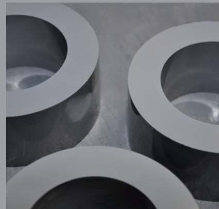
The finished green parts from shaping are waiting for the approval for sintering. This will be given after a positive control of all dimensions according to the drawings, of a test sintering and after the release by the metallurgical production control.
