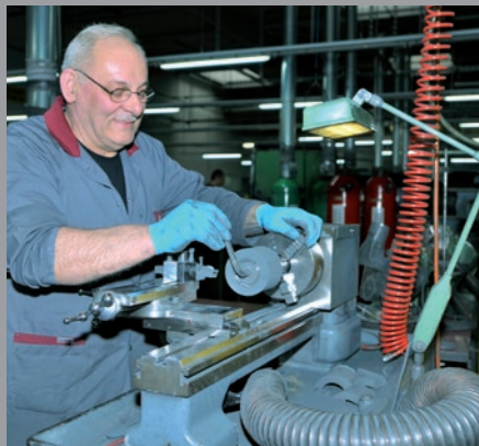
Our mechanics in the shaping department machine the pressed and pre-sintered green blanks on conventional turning lathes or on CNC-controlled machining centers by use of diamond and PCD tools. The precise shaping of the break-sensitive green parts requires a great deal of caution and a good understanding of technical drawings.
